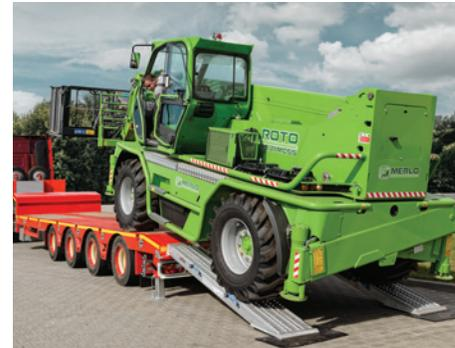
Flip-down and shifted by a hydraulic engine, 3-5 m long or aluminium models added or fixed, 2.4-3 m long.
