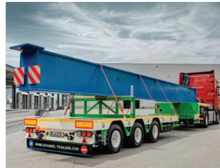
Load trestles are used to level the loading floor with a swan neck. Their number depends on the weight and length of transported elements. It is possible to adjust the shape individually.
