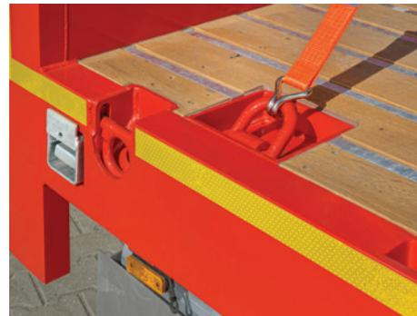
Steel, hot-dip galvanized telescopic arms, retractable in the loading floor and special lashings with a load capacity up to 32 t, with the possibility of storing in the loading floor.
