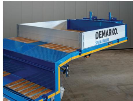
Aluminium side walls, fixed at the front, integrated with a closed tool storage, allow transporting small cargoes or storage of equipment used for loading.
