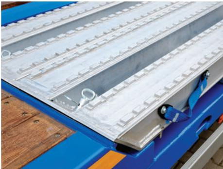
Universal, light and strong aluminium filling for wheel recess allows using the trailer as a typical construction with even a loading floor.
