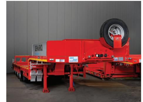
A clamp securing the spare wheel at the front of the semitrailer may hold 2 spare wheels.
