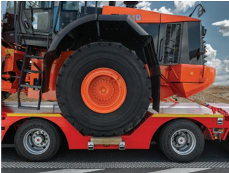
Easy loading of wheel loaders. The dimensions and placing of the recess is optimal for the majority of types and brands of wheel loaders and ensures perfect distribution of the weight between a swan neck and axles.
