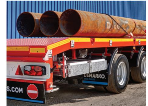
Aluminium ramp basket under the rear cut-out of the loading floor allows for fast and safe transport of additional equipment and increases the loading capacity of the swan neck.
